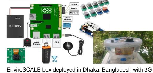
modem and multiple types of gas sensors to monitor air quality
